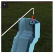
1. Prior to fitting the corner insert the special longer wire tie CRN012, into the corner as indicated
